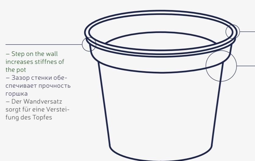
– Step on the wall increases stiffness of the pot
